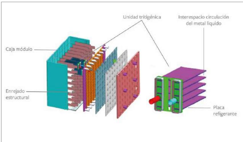
Figura 3.13 HCLL (*Helium-Cooled Lead-Lithium*)
